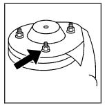
The remote negative (–) terminal, marked GND (–), is located behind the engine coolant surge tank.
